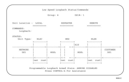
Figure 541-8b. HRX Network Loopback Screen (One HRX)
